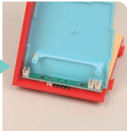
Assemble the ⑦ Circuit Board to the rear side of the Floorboard as shown.
